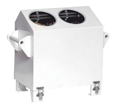
The CBME80B Cloud Ceilometer is a compact and lightweight standalone instrument for measuring cloud base height and vertical visibility.
