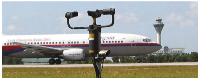
VPF sensors were the first forward scatter sensors to be used in a UK CAA approved RVR system on a CAT III runway.
